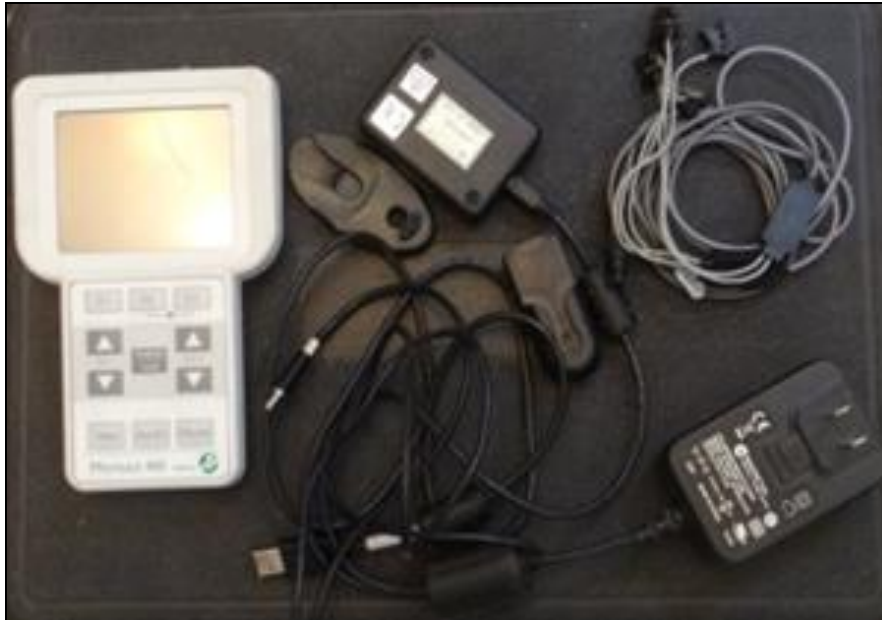
Fig 1: Shows the device system (EMG) Type (Myo trace 400) with the (Bluetooth) transmitter
